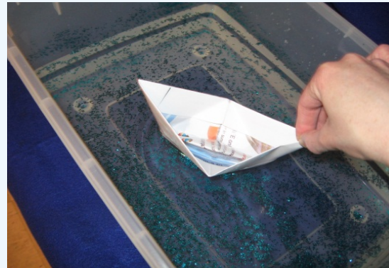
A boat with a bow slices through the water, allowing the boat to move forward more easily.
